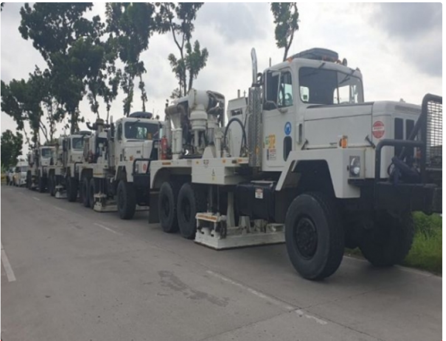
Survey Seismik 2D Vibroseis/foto: dok Pertamina
